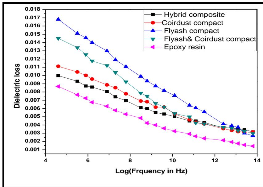
Fig. 9: Variation of dielectric loss with frequency
