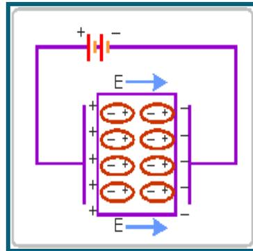
Figure 7: Schematic diagram of the applied electric field for a dielectric
