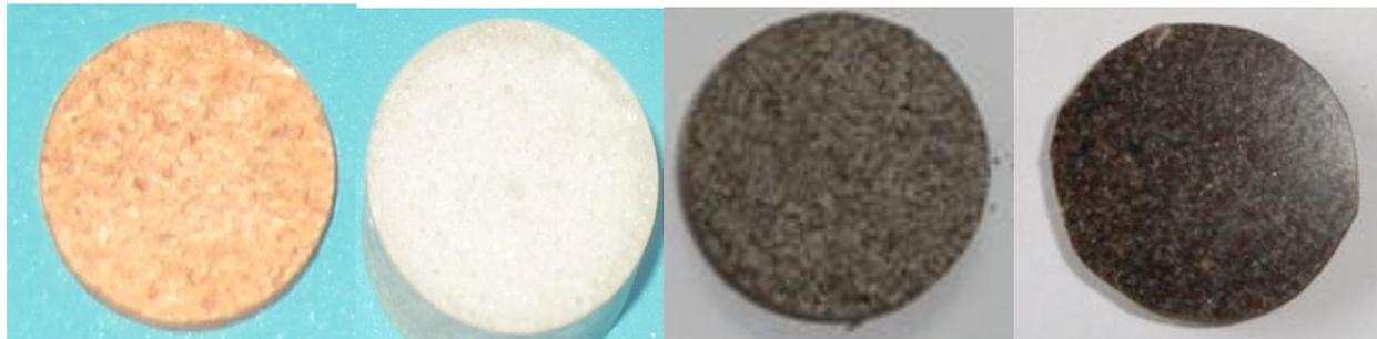
Coir dust compact      Fly ash compact      Compact of Coir dust & Fly ash      Hybrid Polymer Composite
