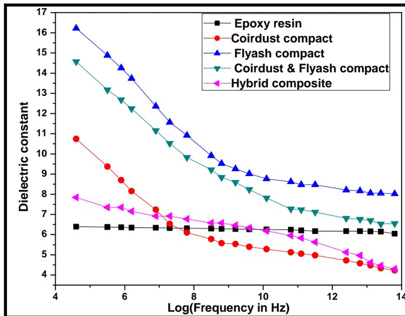
Fig. 8: Variation of dielectric constant with frequency of applied electric field
