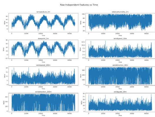
Figure. 4 The raw time-series data for Location 1 is presented before any normalization has been applied. The plot covers the full historical record and includes the eight environmental inputs: temperature, humidity, dew point, and wind speed and direction.
