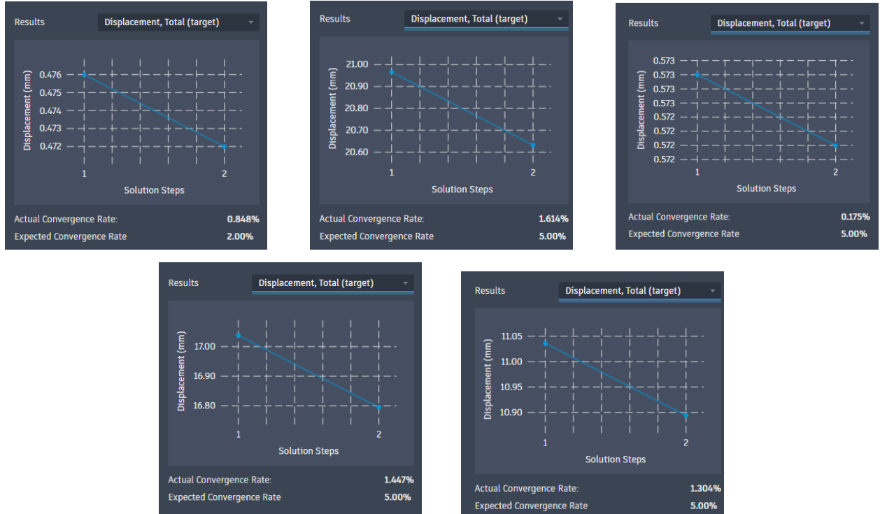
Figure S1. Fusion 360 adaptive-refinement convergence output for the mesh studies summarised in Table S1: semi-spaceframe and ladder frame under torsion (top left, top centre), semi-spaceframe and ladder frame under asymmetric payload (top right, bottom left), and ladder frame under symmetric payload (bottom right). Each plot shows the target displacement across successive refinement steps together with the achieved convergence rate. Numerical values for all six combinations, including the semi-spaceframe symmetric case, are given in Table S1.
