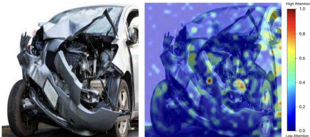
Figure. 5 Attention map of a representative large prediction error by the DINOv2 model. In this example, the attention appears more diffuse and scattered across the image, with less concentration on visually informative damage regions. The model predicted 9,609 USD compared to the ground truth value of 2,652 USD. This example illustrates a case in which the model's attention does not appear to correspond as closely to the regions most relevant to estimating the claim cost.
