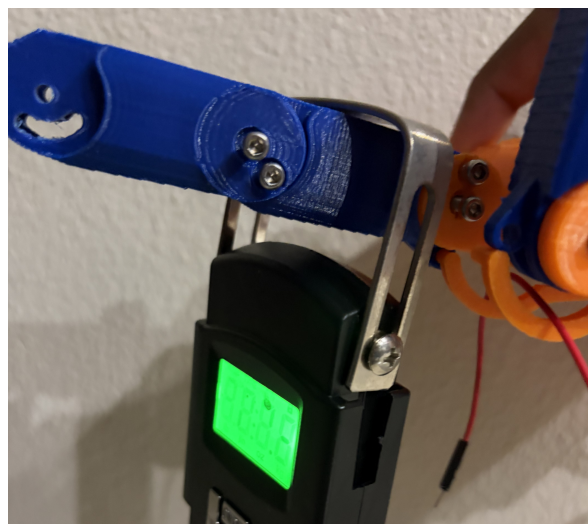
Figure. 10 Data collection is set up for linkage-driven design. The mass of the digital luggage scale was included in the overall weight. Exact mass was found by looking at the product page, and it was fixed by bolting a screw through the scale to the finger.
