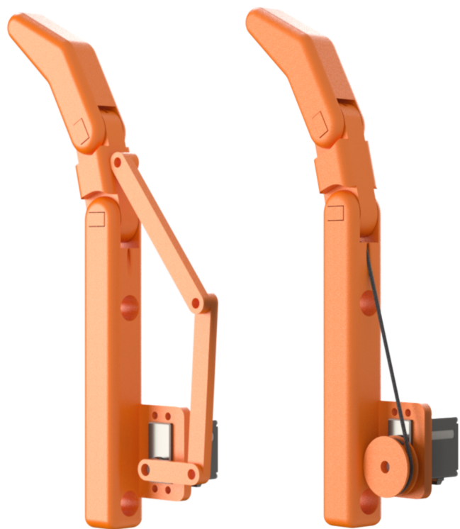
Figure. 3 Side-by-side of linkage (left) and tendon (right) drive single finger prosthetics. The diagram shows the comparison between the linkage-driven and tendon-driven designs. Each design has identical geometry with the inclusion of specific hardware for each actuation type.
