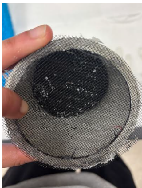
Appendix 8 : Double layered nylon mesh was able to capture some microplastics in the small triangular overlaps between the first and second layer of mesh
