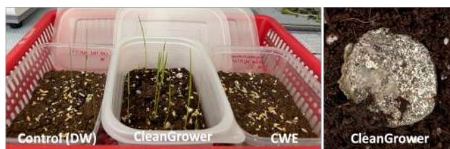
Fig. 19 Growth of rice in soil remediated by CleanGrower (Control = Soil with DW, Device = Soil with CWE and CleanGrower, CWE = Soil with CWE)
