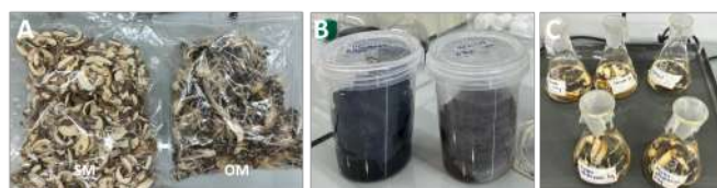
Fig. 6 Removal of heavy metals from CWE using mushrooms (A. Dried shiitake mushrooms (SM) and oyster mushrooms (OM), B. Navy CWE and Brown CWE, C. CWE with mushroom on a shaker)
