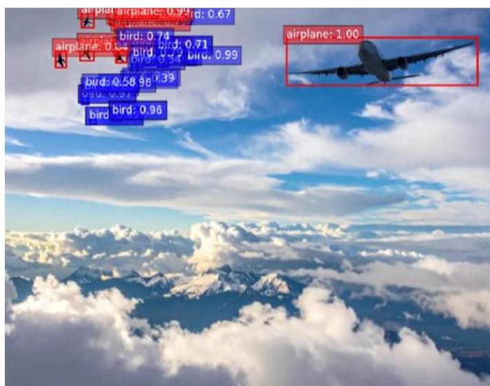
Fig. 4 Qualitative examples for error analysis. (a) birds inaccurately detected as airplanes (b) the central plane is detected as a separate object
