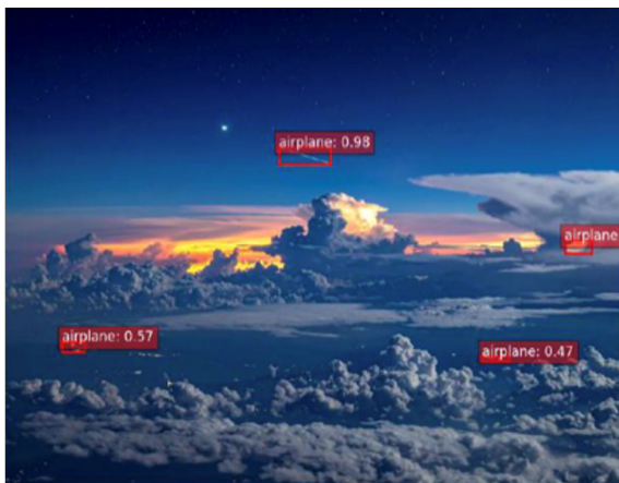
Fig. 5 Qualitative examples for error analysis. (a) star falsely detected as a bird (b) cloud falsely identified as airplane (c) cloud streak falsely identified as airplane (d) airplanes not detected at all
