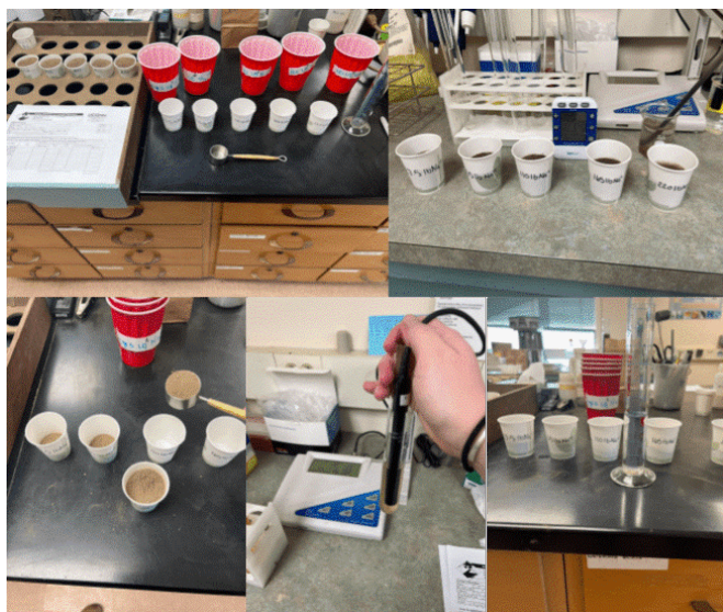
Fig. 4 The method and procedure by which the soil nitrogen test was taken at the UCONN soil nutrients laboratory, illustrating the method used for sample collection, chemical preparation, and measurement of nitrate concentration.
