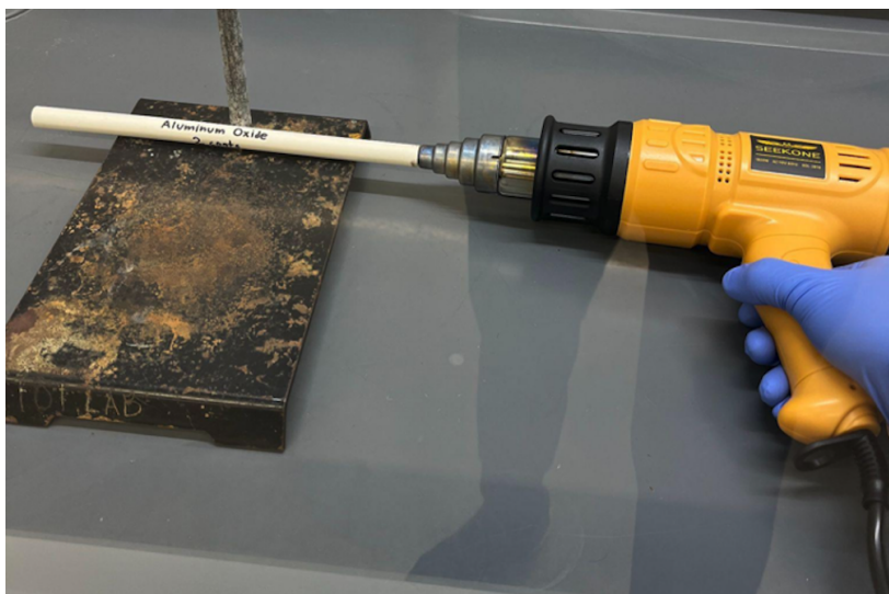
Fig. 2 The ceramic rod is put onto the retort stand, with the heat gun placed at one end of the rod. This setting is a simplified system designed to mimic the heating and air turbulence generated in an aircraft engine.
