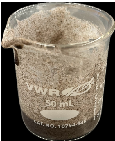
Fig. 1 The aluminum oxide mixture consists of aluminum oxide powder, glue, and water. This formula is used to produce an aluminum oxide coating for the heat insulation experiments.
