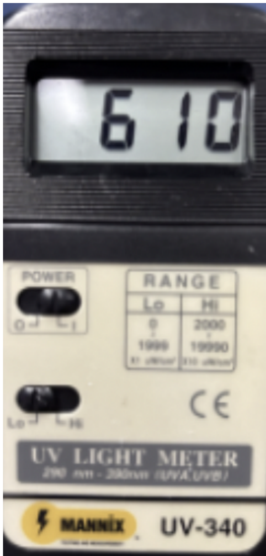
Fig. 3 UV light meter confirming UV-A irradiation of 610 \mu W/cm^2 (Photos by authors, 2025)
