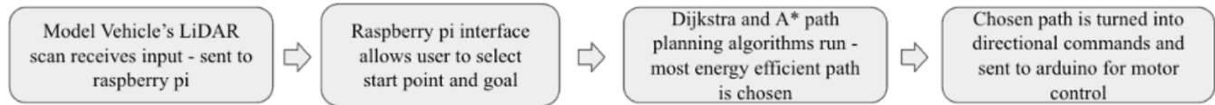
Fig. 1 Flowchart representing full pipeline of code from LiDAR scan input to drive commands being executed.
