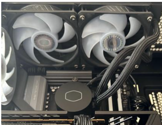
Fig. 3 Liquid Cooler used in the experiment and its various components. The water block, integrated pump, radiator and fans are seen in this picture.
