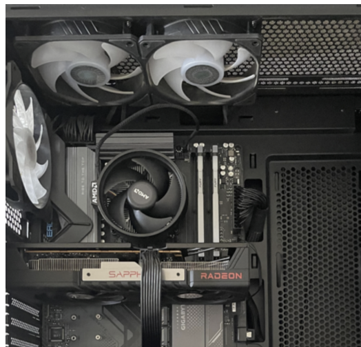
Fig. 5 This is the picture of the Consumer PC that was used for the experiment. This figure shows the air cooling leg of the experiment and the components such as the RAM and the graphics card.
