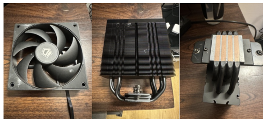
Fig. 1 The components of an air cooler . (a) Fan that blows air over the heatsink for dissipation of heat, (b) Heatsink- the image showcases its fins, (c) Heat pipes-the image showcases the copper heat pipes which help take heat away from the CPU to the heatsink.
