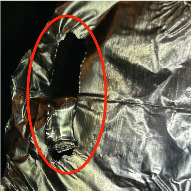
**Fig. 5** Small tear due to adhesion, but likely not from a cold weld.
