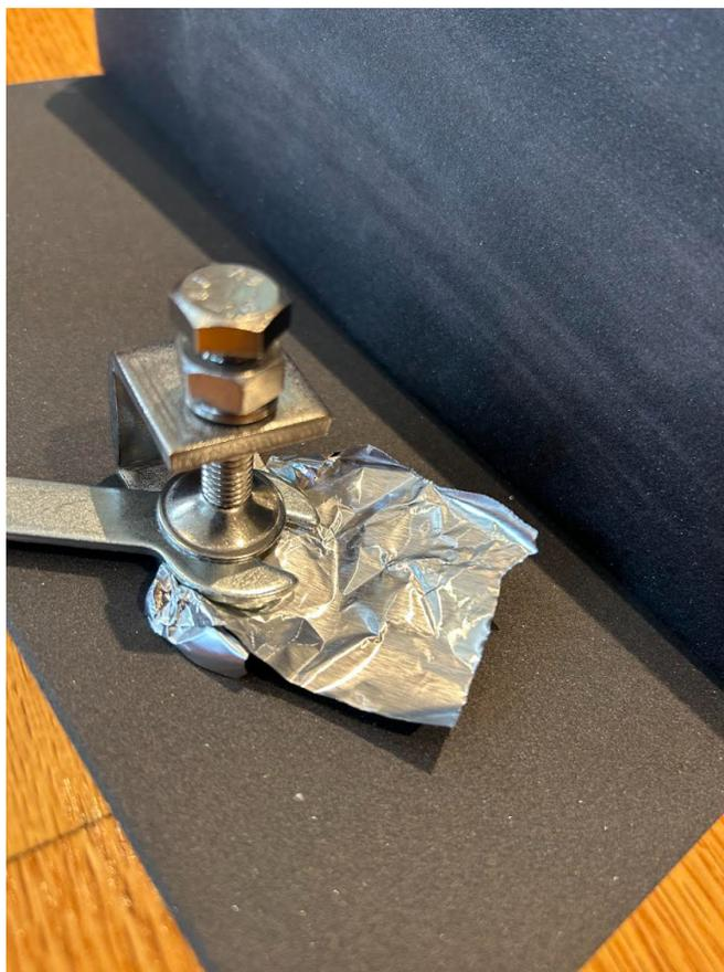
**Fig. 3** A small C-clamp was used to apply continuous pressure to the aluminum foil. A wrench was placed between the C-clamp and the aluminum foil as a flat surface to provide even pressure distribution.
