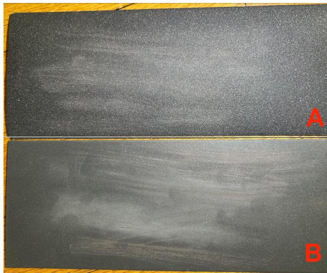
**Fig. 4** Two grits of silicon carbide sandpaper were used: (A) coarse P320; (B) fine P800. Both show silver and bronze streaks from worn aluminum and copper.
