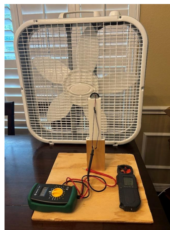
Fig. 4 Wind turbine setup
