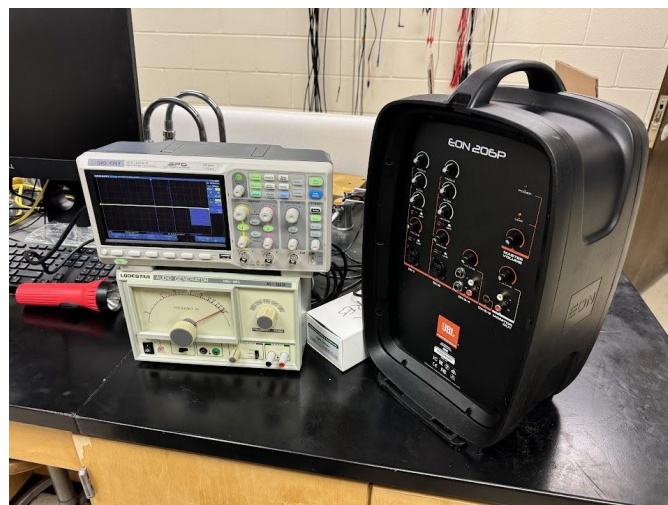
Fig. 5: The picture displays the oscilloscope (top left) plugged into a wave generator (bottom left). The wave generator also plugs into the amplifier (on the right).
