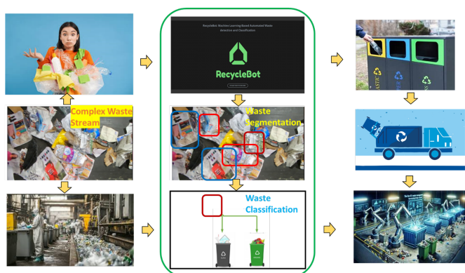
Figure 9: Illustration of the two-step AI-enabled pipeline used in RecycleBot. The process involves initial segmentation of waste objects using a ViT-based model, followed by classification into recyclable or organic categories using a VGG16-
