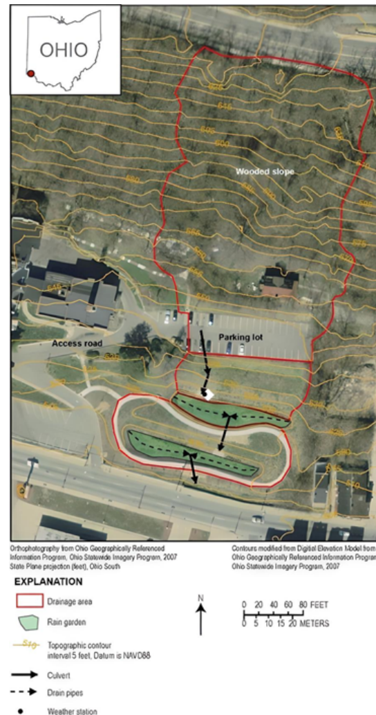
Fig. 2 Figure depicting the St. Francis, Cincinnati green infrastructure network, including rain garden, drainage area, and conveyance infrastructure 3 .
