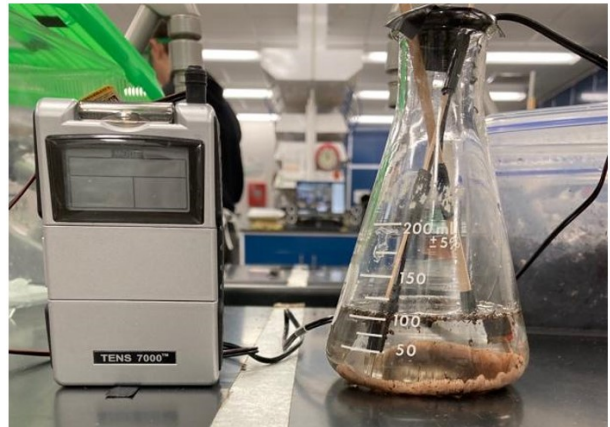
Fig. 6 Electrical Stimulation Set up (Photo by authors)
