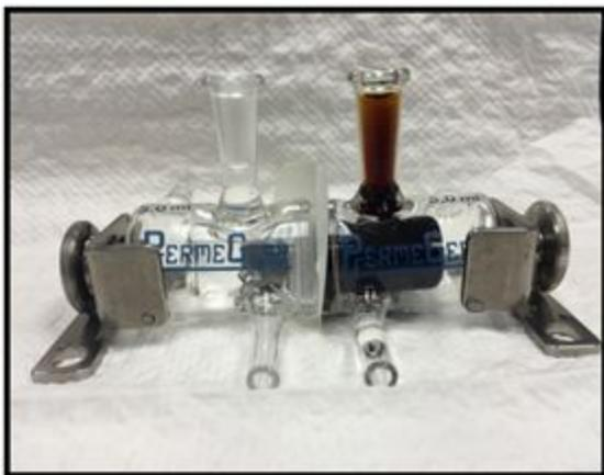
Figure 4. Apparatus used for salt rejection testing. A) Two halves of diffusion cell with clamp, B) fully assembled diffusion half-cells with stir bars in each half and CNT membrane positioned
